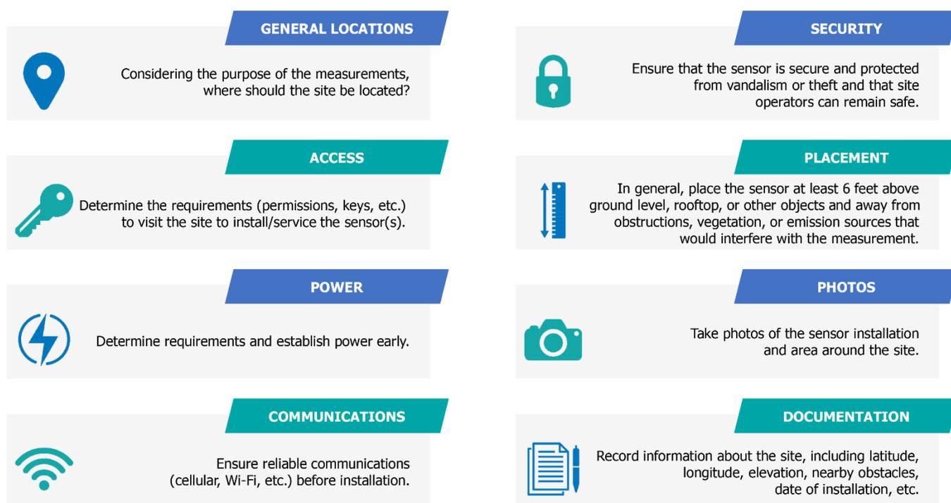
**Figure 3-7. Logistical Considerations and Tips for Installing an Air Sensor**
